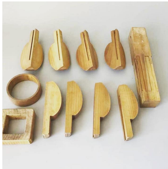
Image 6. Deconstructed Kigata Banko mould.
