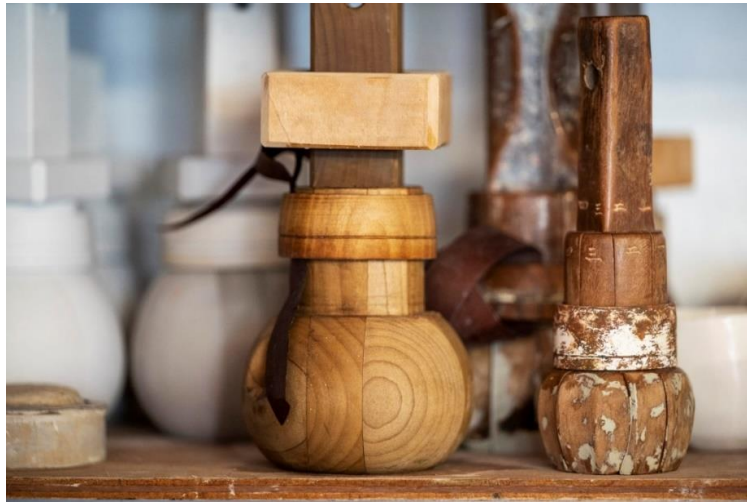
Image 5. Constructed kigata Banko moulds
