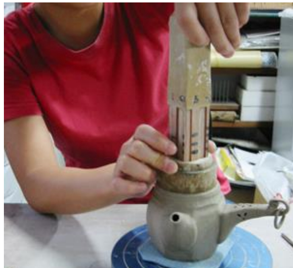
Image 8. A mould being removed
